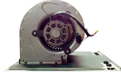
If there is evidence of dirt or dust build-up in the evaporator motor or blowers, they should be cleaned either by vacuum cleaning (if working in an apartment) or by removing the unit to a workshop location and cleaning with compressed air.
