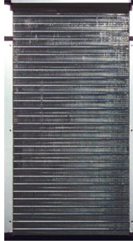
Check the coil for cleanliness and uniformity of fins. If the coil is dirty, vacuum clean with a soft brush attachment. This is the only form of cleaning that should be carried out within an apartment. If the coil requires additional cleaning, the unit must be removed and cleaned using compressed air and/or washed. These operations MUST be carried out in a facility properly equipped to handle this type of work in a safe and professional manner.
